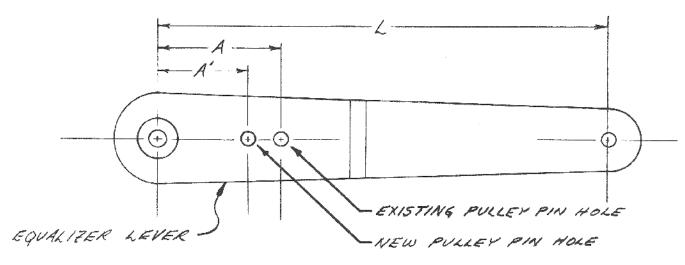
OLD MECHANICAL ADVANTAGE =  $\frac{L}{A}$ \* NEW MECHANICAL ADVANTAGE =  $\frac{L}{B}$
