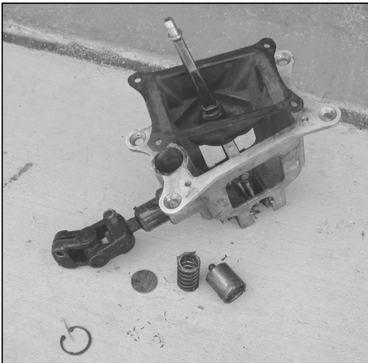
With the unnecessary parts removed, the shifter is ready to go
