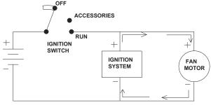
Engine Running On. Ignition Switch in the OFF Position. Current flowing thru the Ignition System from the Fan Motor. Polarities are shown. This occurs because the Fan Motor acts as a generator while the fan is running down. Occurance depends on Fan capacity and Ignition System type and power requirements.
