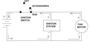
Normal circuit confiruration. Ignition Switch in the Run Position. Current flowing thru the Ignition System and thru the Fan Motor. Polarities are shown.
