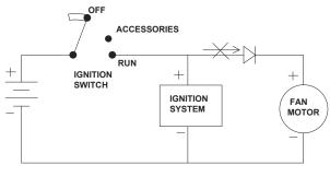
FIX #1: Insert a diode in the power lead to each Fan. Engine Run-On Prevented. Ignition Switch in the OFF Position. The diode will block current flow thru the Ignition System from the Fan Motor. Polarities are shown. The diode will allow the fan to run when the ignition switch is in the Run position. Fan voltage will be reduced ~0.7V from normal.
