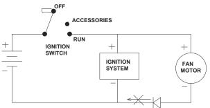
FIX #2: Insert a diode in the ground lead from each Fan. Engine Run-On Prevented. Ignition Switch in the OFF Position. The diode will block current flow thru the Ignition System from the Fan Motor. Polarities are shown. The diode will allow the fan to run when the ignition switch is in the Run position. Fan voltage will be reduced ~0.7V from normal.
