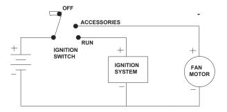
FIX #3: Reassign the Fans to the Accessories bus. Engine Run-On Prevented. Fans connected to the Accessories position of the Ignition Switch cannot provide current thru the Ignition System. Fans will operate normally in the Accessories and Run positions of the Ignition Switch but will be disabled in the Start position. All wiring changes can be made at the Fuse Block. No Additional components or wiring required.
