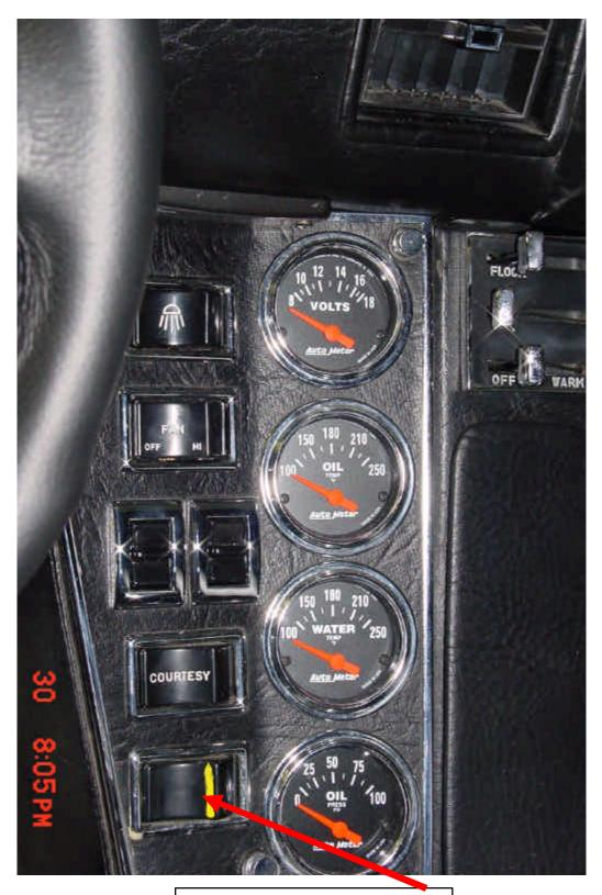
Switch To activate accusump. Yellow line means powered on.
