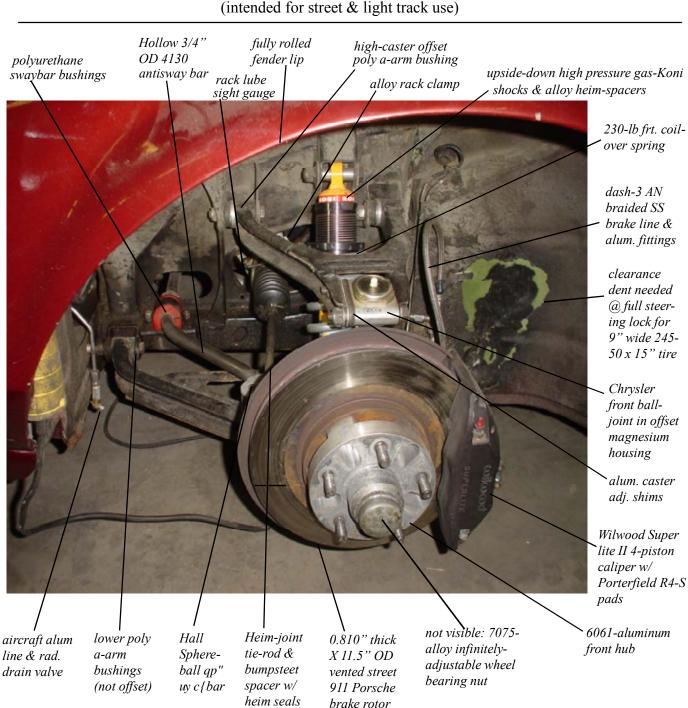
DRIVER'S SIDE OF OUR '72 L- MODEL PANTERA FRONT SUSPENSION (intended for street & light track use)
