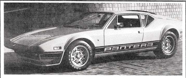
FENDER FLARES These fender flares add the perfect performance feel to the Pantera. Pop riveted for easy installation. Allow the use of wider wheels---but look great on the car with normal wheels and tires.
