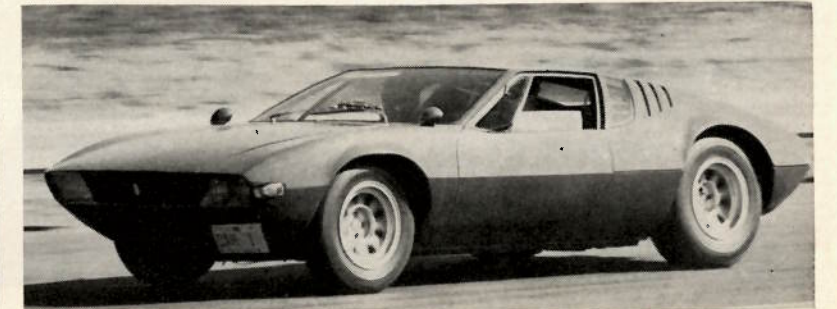
The Mangusta cornered flatly, left, mainly because of a suspension which resembles a modern-day race car. Below left, there was plenty of power and fast acceleration with modified Ford engine. Although aerodynamic design made front end lift at high speed, below, car was stable. Bottom left, like most deTomaso products, making repairs isn't easy, as close quarters in engine compartment disclose. Bottom right, a quick check by SCG opens many doors.
